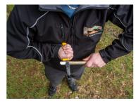
Alternatively use the forearm cut. Again, remember the knife remains static whilst pulling the workpiece.
