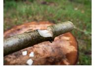
8. Using the chest lever cut, start removing the wood at the end going in the ground to form a blunt point. Again, remember the knife remains static.
