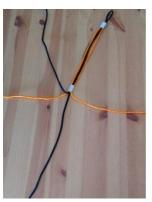
7. Take one strand and lay it over the strand clockwise from it, to form a loop. Take the next strand and do the same thing. Repeat this with the third strand and finally, lay the fourth strand over the core of the fender and down through the first loop. Pull each strand tight to secure the ends in the crown. This is illustrated below.
