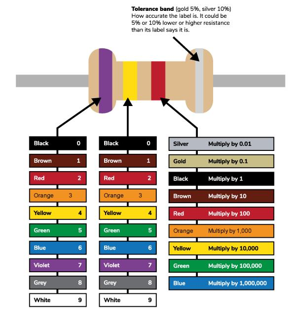
Most resistors are labelled with four coloured bands.
