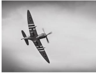
Monoplane – aeroplane with one pair of wings.
