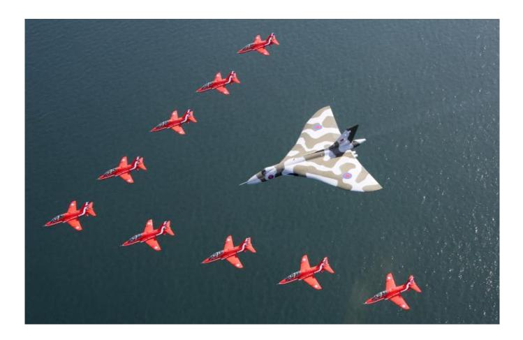
Tailless – an aircraft that has no tail and no other horizontal surface besides its main wing. Delta wing - a wing shaped in the form of a triangle.
