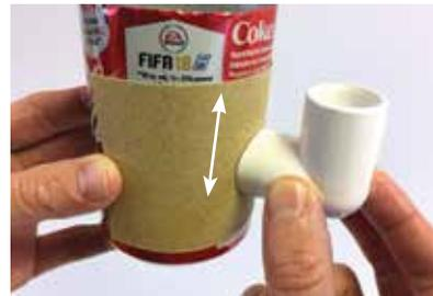
**2** Using the other drink can, wrap sandpaper around it and press the 22mm PVC pipe elbow against it. Sand away the pipe until the shape of the can is formed into the end of the elbow.
