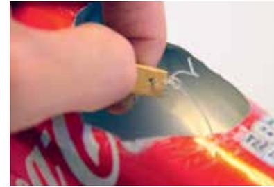
**16** Tie the fishing line from the displacer onto the bottom hole of the crankshaft. This must be tied ensuring that the wire wool does not clash with the bottom of can 1 or can 2 when in motion.
