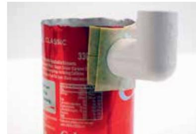
**3** Using double-sided tape, cover the formed end of the PVC pipe, leaving sufficient overlap to seal to the can. Using the craft knife, cut the inside of the double-sided tape to clear the pipe, leaving a seal on the edge. Adhere the elbow facing upwards onto the can. Its position should be about 10mm below the top.
