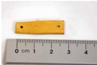
**10** Make the connecting rod: cut the lolly stick down to approximately 25mm in length. Drill two holes at either end.
