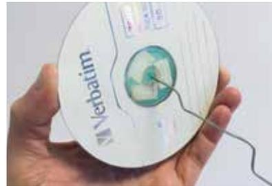
**19** Push the flywheel onto the crankshaft, positioning the CD first.
