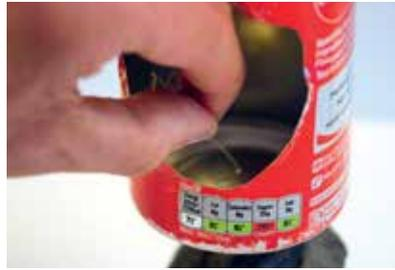
**14** Being careful of any remaining sharp edges, insert the fishing line connected to the displacer through the pierced hole in can 2.
