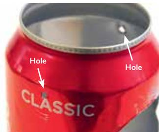
**7** Using the drawing pin, pierce two holes directly opposite each other at the top of the can. Make another small hole in the base of the can, as central as possible.
