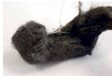
**12** Make a displacer: Cut a piece of steel wire to approximately 25mm in length and tie a length of the rigid wire onto the centre of the steel wire. Wrap wire wool around the ends of the steel wire to create a small cylinder, keep adding wire wool until the outer shape is slightly smaller than the inside of Can 1. When complete the displacer should be able to move up and down inside the cut can using the rigid wire.
