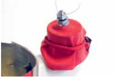
**13** Fit the balloon over the PVC pipe elbow and secure it in place using the end of the balloon like an elastic band.
