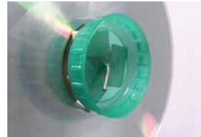
**20** Place a small section of double-sided tape inside the milk bottle cap and then bend the end of the crankshaft inside the cap and press it against the tape to secure it. Trim the crankshaft if it is too long.
