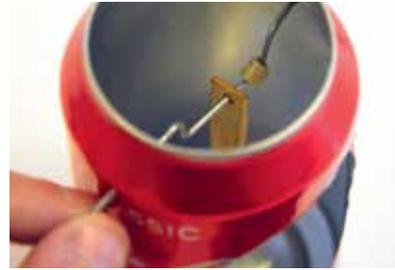
**15** Loop the lolly stick onto the crankshaft and position the crankshaft through the two holes in can 2.
