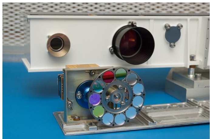
Above: Part of PanCam, a camera designed for the Mars Rover which is being built in the UK. The filter wheel in front of it can move. This allows the machine to take pictures of Mars, using the different filters to allow different things to be seen. Source: MSSSL
