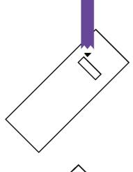
4. Drill holes inside the marked rectangle to create the slot and use a saw or rasp to clean it up and make it square.
