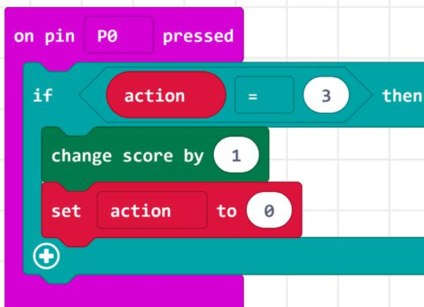
**7** Test your game. When a **0** appears on the display, tap the free end of the crocodile clip lead on the **0** pin. If you don't have a crocodile clip lead, you can hold the **GND** pin with one hand and then touch and release the **0** pin with the other hand. This works because your skin is conductive – if it doesn't work, you might need to drink more!
